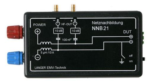
Measurement of conducted disturbance emissions
